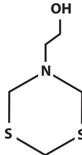
Figure 3. Dithiazine chemical structure. During scavenging, the monoethanolamine groups are substituted by sulfur from hydrogen sulfide. The free monoethanolamine can participate in further scavenging.
